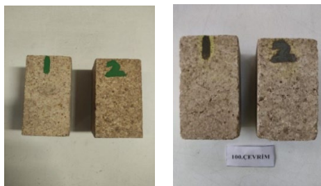
Figure 4. Brick images before and after thermal shock test (Number 1 Trial Brick, Number 2 Standard Product)
